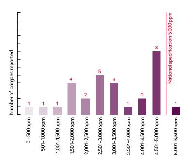
Figure 7.3 – Diesel imports in Ghana by sulphur content (2014)
