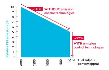
Emission control technologies become fully effective only at 10–15 ppm or less. This is why it is impossible to clean the air without first removing sulphur from fuels. | SOURCE: UNEP and ICCT
